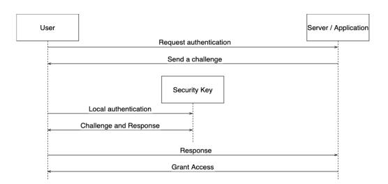
Figure 2.4. Security Key challenge response, basic authentication schema.
