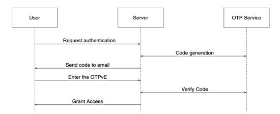
Figure 2.1. One-Time code via Email, basic authentication schema.
