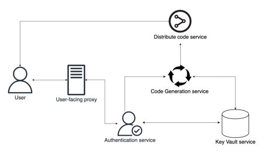
Figure 3.2. Passwordless architecture with One-time codes.
