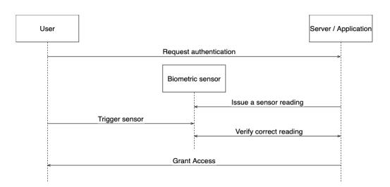
Figure 2.3. Biometric reading, basic authentication schema.
