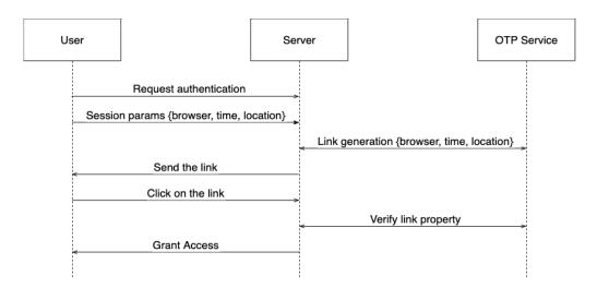
Figure 2.2. Magic Link via Email, basic authentication schema.
