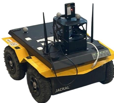
**Figure 4.2:** Jackal UGV configuration used for all the experimental tests.
