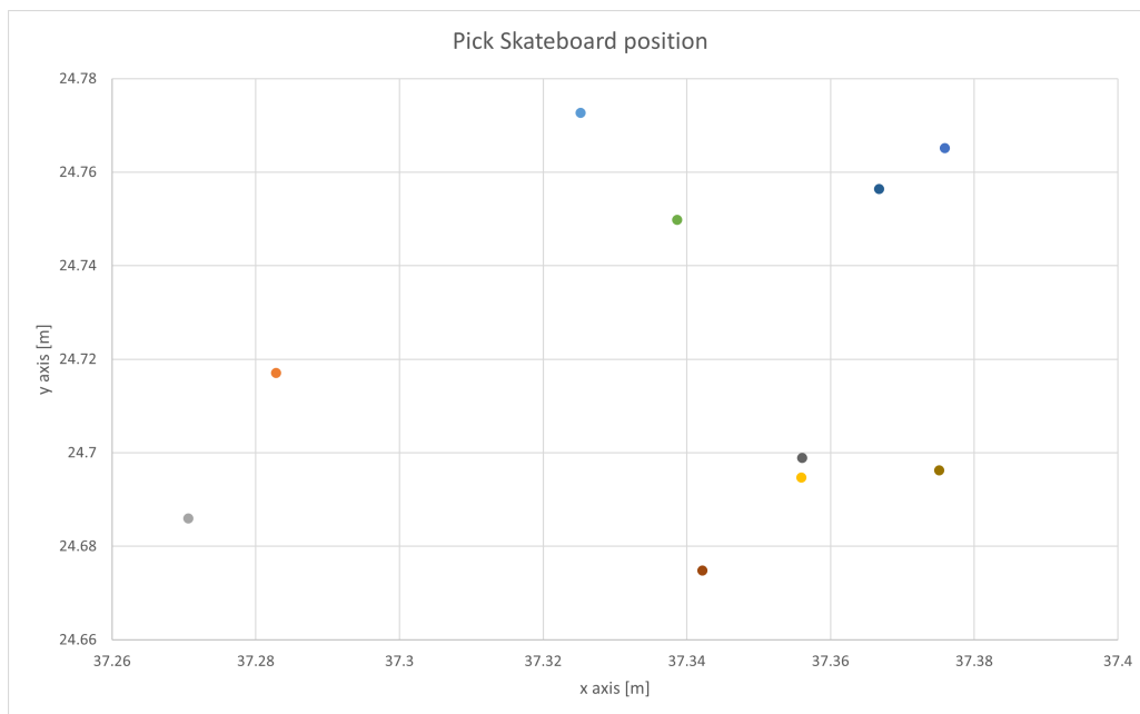
Figure 19: Ten arrival points of the MIR100 in the Skateboard picking point in the Initial Warehouse.
