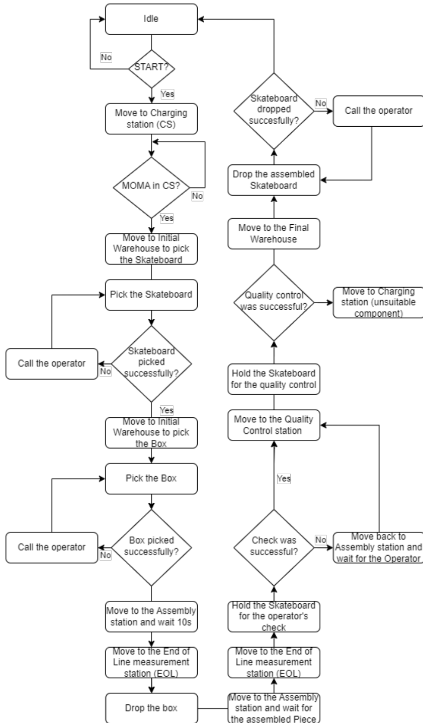
Figure 76: Flow chart of a MOMA's cycle of production.
