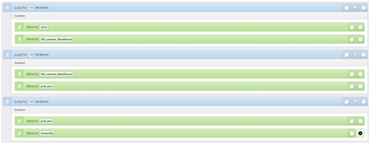
Figure 18: Script for three stations to study the accuracy of the MIR100.
