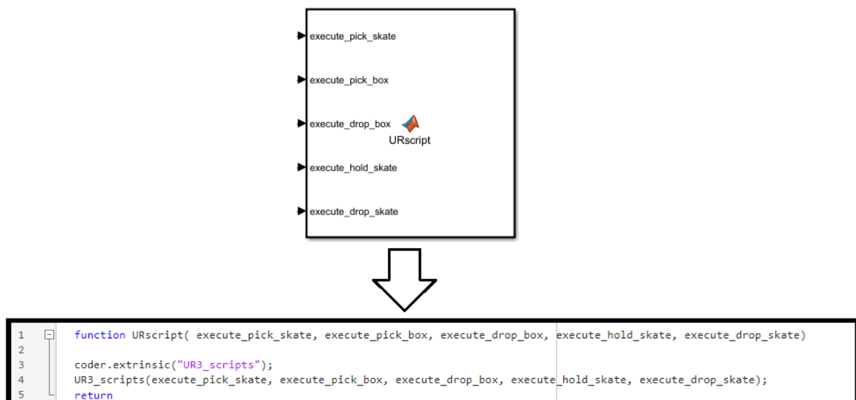
Figure 87: 'URscript' MATLAB function block calling the MATLAB function to control the UR3.
