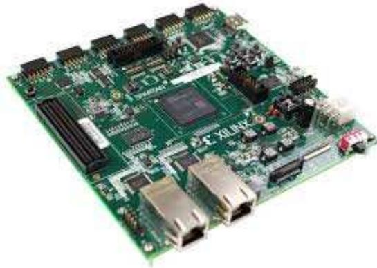
**Figure 1.3:** A Spartan®-7 SP701 FPGA
