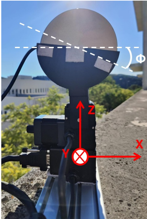
Figure 6: PTU pan angle and LiDAR's internal spin motion angle
