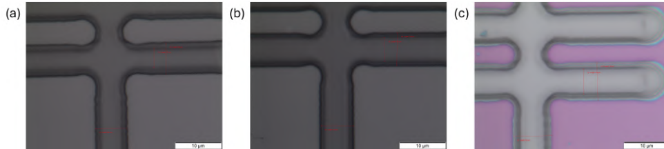
Figure 3.6: Comparison between different developing times: (a)50 s, (b)60 s and (c)70 s. As time increases, one can appreciate higher curvature in the Hall bar geometries, meaning that the development solution has consumed the hard PR more. Darker areas in a),b) and grey areas in c) are substrates covered by photoresist, while the rest of the pictures show a nude substrate.
