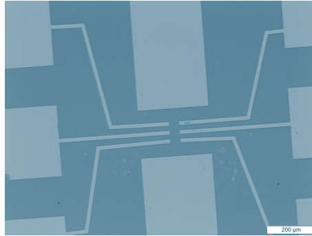
Figure 3.7: Optical microscope image of the etched profile. Despite being only a few tens of nanometers, the Hall bar pattern etched by CHF_3 and Ar gas is perfectly visible and clearly stands out from the PR coated substrate.
