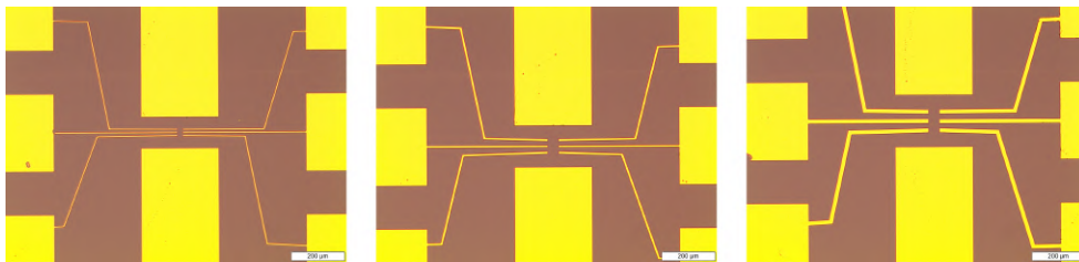
Figure 3.9: Picture of the patterned chromium-gold contacts after lift-off. The optimized recipe succeeded in obtaining a clean set of devices.
