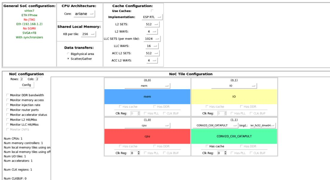
Figure 5.12: SoC design in the ESP GUI with the hierarchical architecture of the 2D-Conv accelerator.
