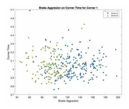
Figure 5.2: Comparison of Brake Aggression for Drivers A and B on Corner 1.
