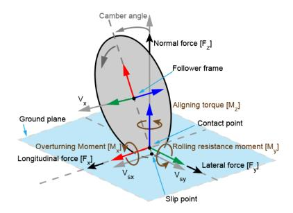
Figure 2.1: Forces acting on a tire.
