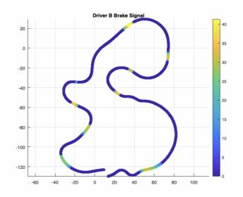
Figure 5.15: Braking zones of Driver B on track layout.
