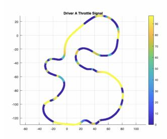
Figure 5.16: Acceleration zones of Driver A on track layout.
