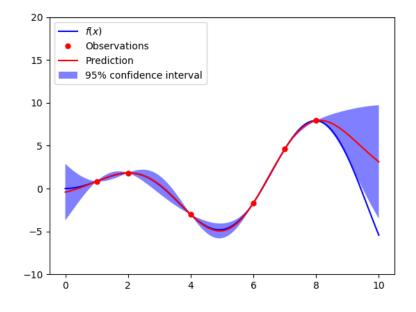
Figure 2.7: Visualization of the working principle of GPR by Subhasish et al.
