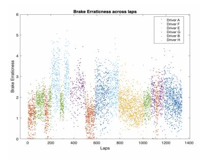
Figure 5.3: Brake Errationess data points per driver.
