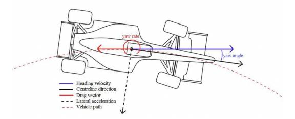
Figure 2.4: Forces acting on a Formula racing vehicle.
