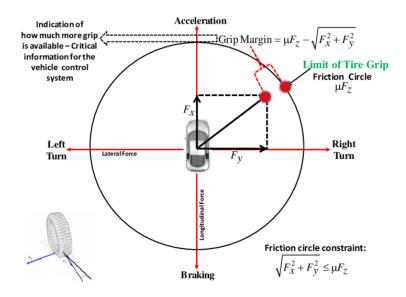
Figure 2.2: Traction circle details by Singh et al.
