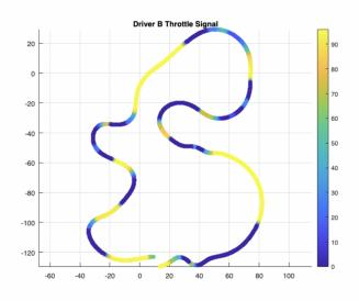
Figure 5.17: Acceleration zones of Driver B on track layout.
