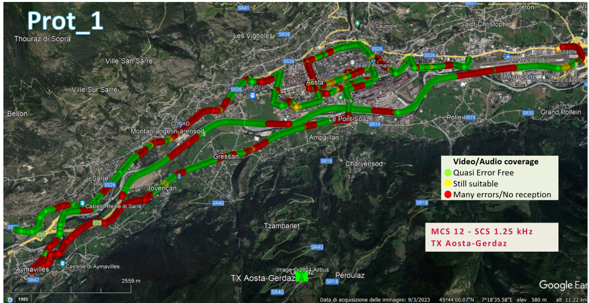
Figure 4.4: Map showing video/audio coverage during real-world testing with Prototype 1 (Prot1) in Valle d'Aosta. The map illustrates the impact of the noise threshold modification, with areas marked as 'Quasi Error Free' (green), 'Still Suitable' (yellow), and 'Many Errors/No Reception' (red) representing varying levels of reception quality.
