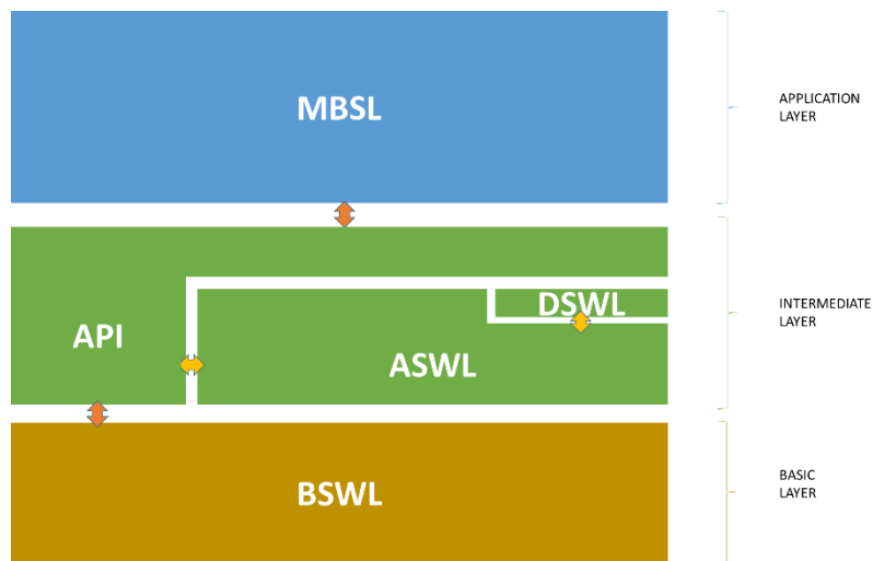
Figure 3.2.2 - HDS9 SW architecture layers
