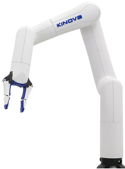
Figure 5.1: Kinova Gen3Lite 6 DOF from [32]
