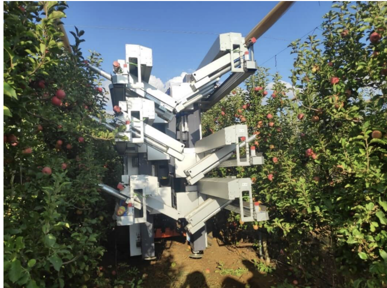
Figure 2.3: Representation of the 12 arms FFRobot from [10]
