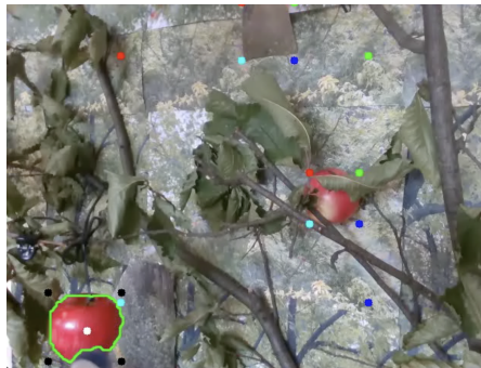
Figure 6.14: View from RealSense for Test n. 1 and selected target with IS model
