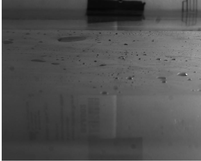
Figure 9: Picture of a floating elastic PDMS membrane, taken from the sequence of images in which we apply a pulse to its surface. We voluntarily added droplets on the surface of the membrane to add texture, for PIV analysis.
