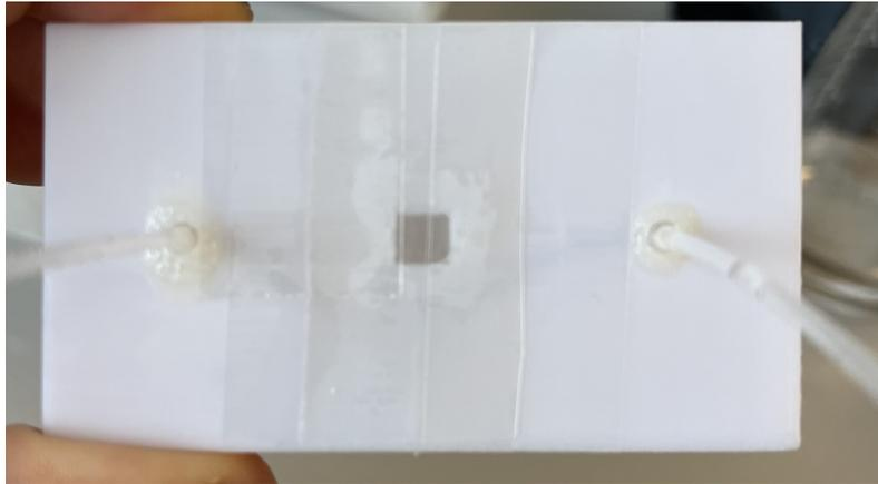
Figure 7.9: Sealing test to close the organoid chamber.
