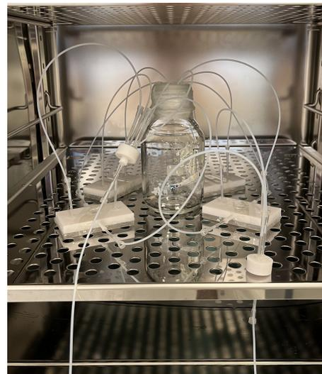
(b) Loaded devices, flow splitters and bottle to collect the output, all connected.
