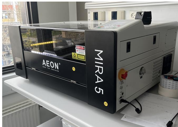
Figure 5.1: AEON MIRA5 CO<sub>2</sub> Desktop Laser Cutting Machine.
