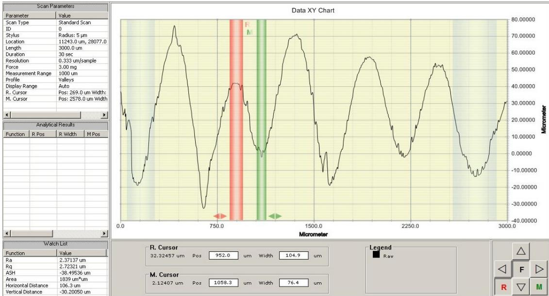
Figure 5.17: Measurement in the center of direction B, without the edge, of the square structure in section 2: random peak height =  $30.2\mu\text{m}$ .
