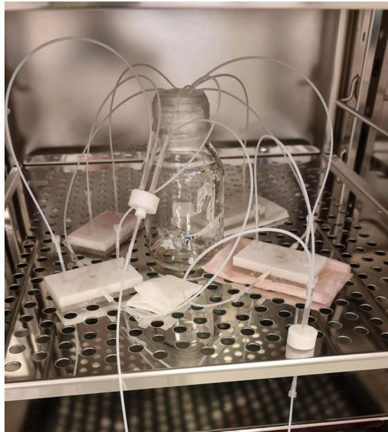
Figure 8.5: Failed experiment with leakages and no waste collected in the output bottle after 2 days and a half of operation.
