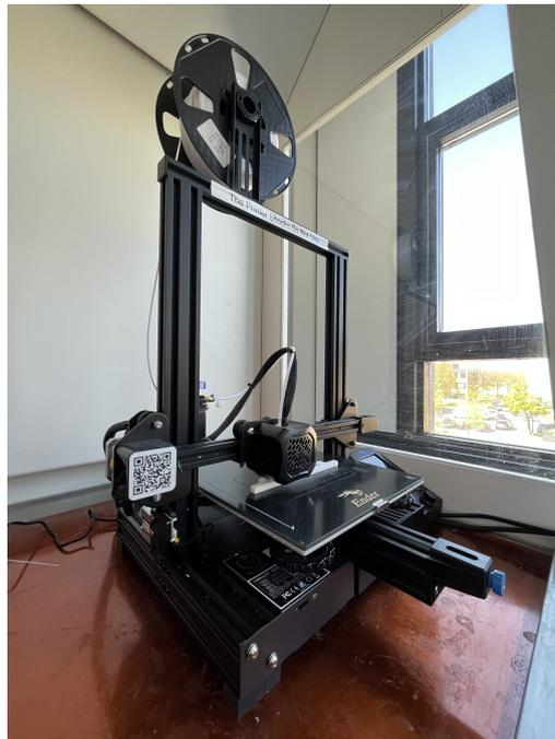
Figure 6.1: Creality Ender-3 V2 filament 3D printer.
