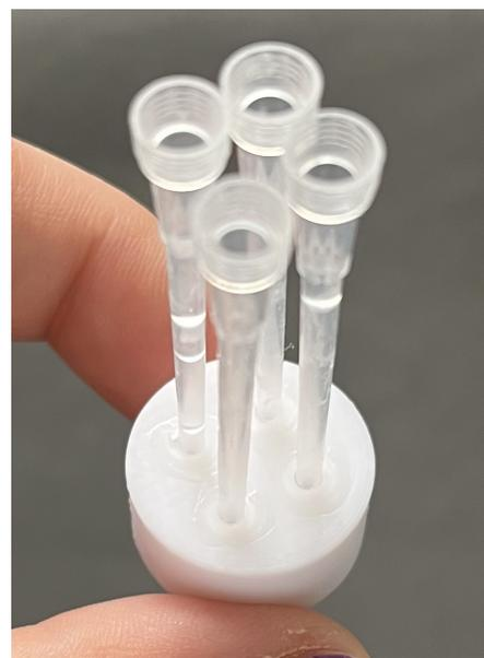
(b) Flow splitter from the bottom.
