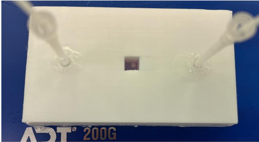
Figure 8.2: Organoid inside of the central chamber of the chip. The pink colour is due to the medium colour.
