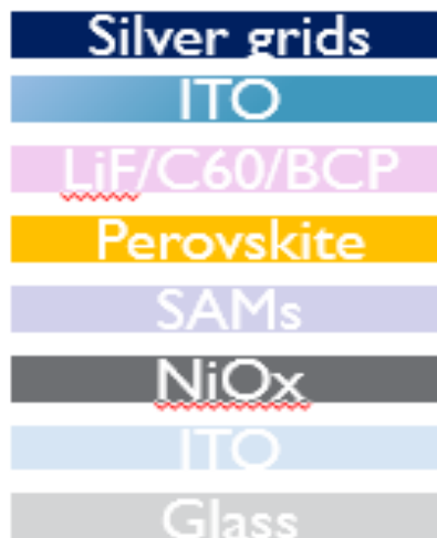
Figure 2.12: Semitransparent perovskite cell stack design.
