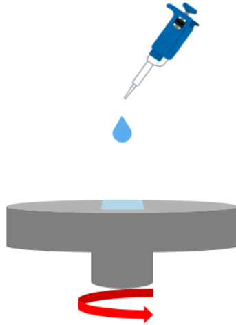
Figure 2.6: A schematic illustration of spin coating process.
