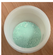
Figure 3.7: NiAlTi photocatalyst in pulverized form: it is possible to notice its characteristics clear green color.
