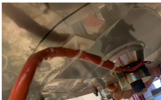
Figure 3.4: Piezoelectric element under the cylindrical vessel, used to induce ultrasounds.
