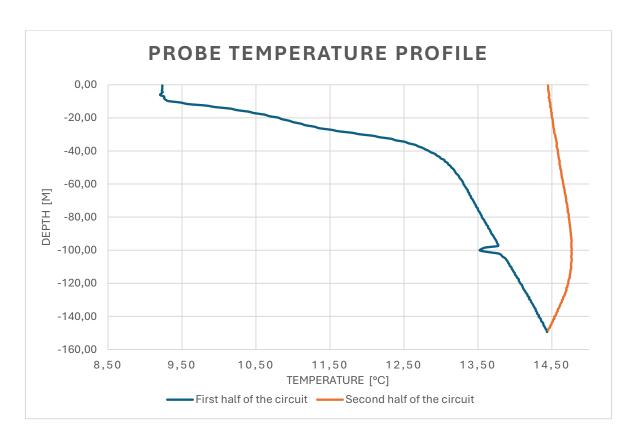
Figure 16 Temperature profile of two half of the circuit
