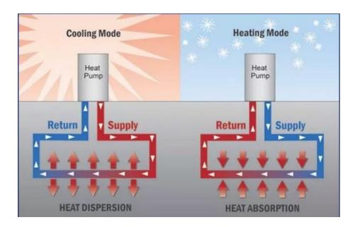
Figure 7 heating and cooling mode operation
