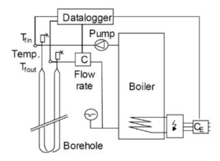
Figure 18 Scheme of operation of the TRT
