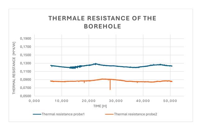
Figure 20 Thermal resistance of the probe with respect time
