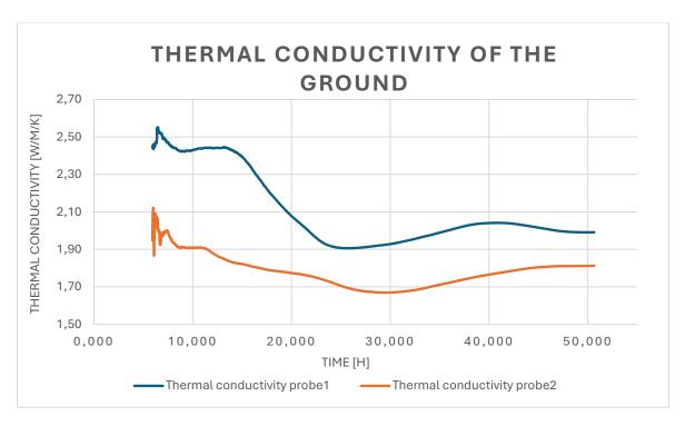
Figure 19 Conductivity of the ground with respect the time
