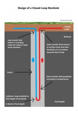
Figure 8 Design of a closed-loop borehole
