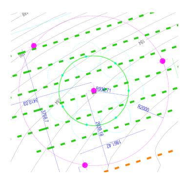
Figure 38 Boreholes layout of the BTES
