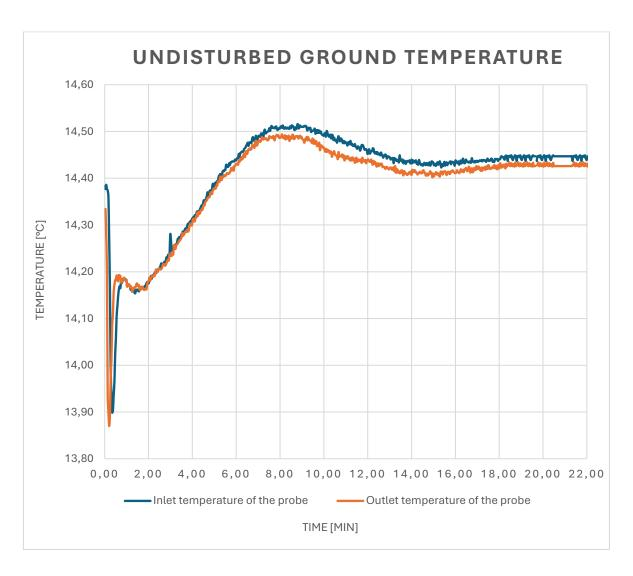
Figure 17 Undisturbed temperature of the ground
