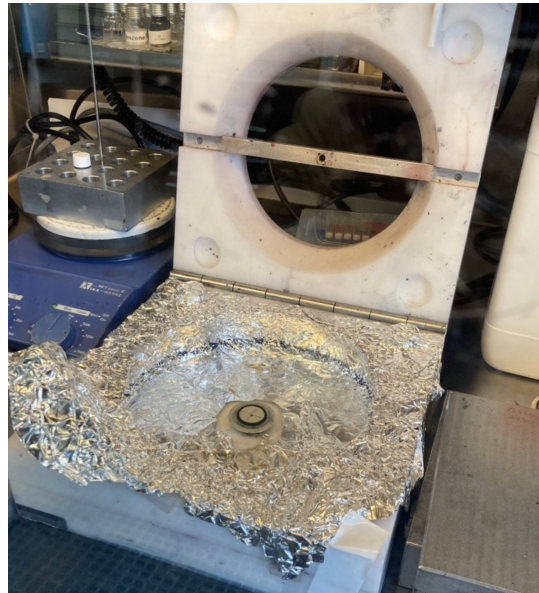
Figure 5.3: Spin coater used for depositing the charge selective layers HTL and ETL, as well as the absorber layer.
