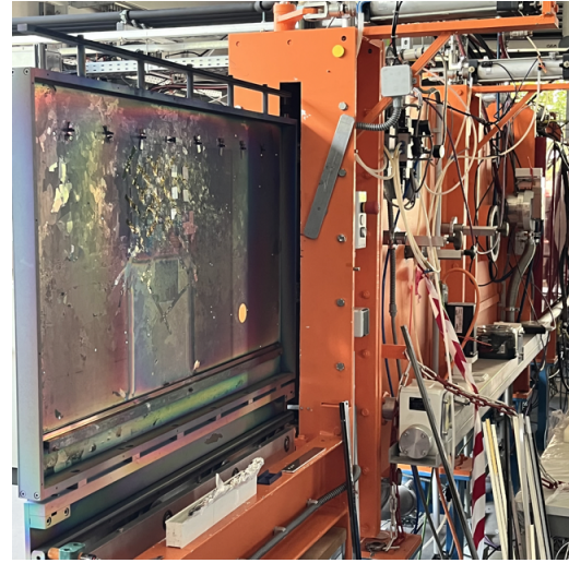
Figure 5.2: Picture of the sputtering process, displaying the equipment used to deposit the layers of the back electrode on the glass substrate.
