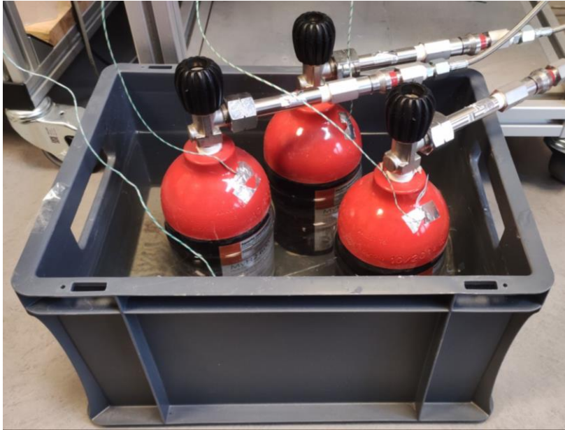
Figure 21: Canisters inside water
