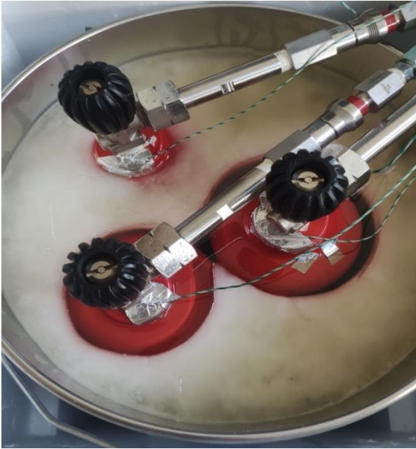
Figure 27: Canisters into coconut oil after desorption
