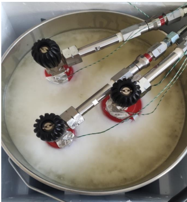
Figure 26: Canisters into coconut oil in solid state
