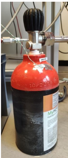
Figure 12: Thermocouple on the storage surface
