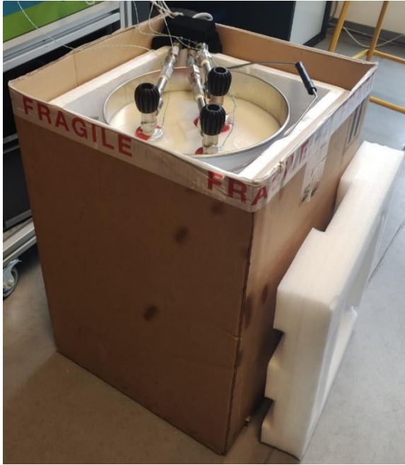
Figure 25: Insulated canisters into coconut oil
