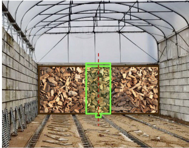
Figure 7.1: Overlay of the woodchip pile and meshgrid dimensions on the real case study plant. The green highlight shows the section modeled in the simulation
