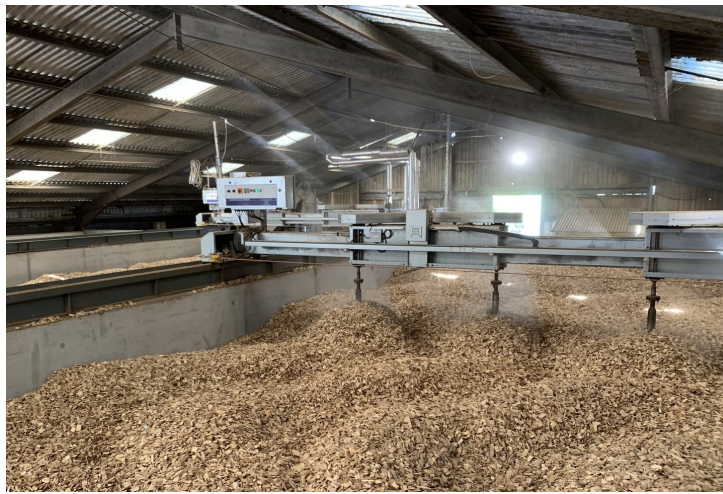
Figure 2.4: Picture of an open air drying plant with mechanical turning [8]
