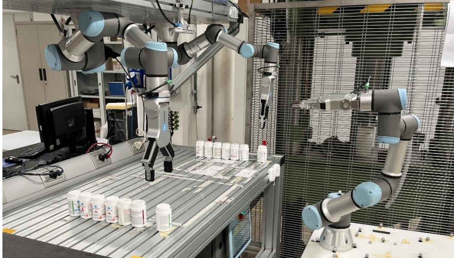
Fig 19. Set up of the Application in the Laboratory, with the addition of the third robot performing the dynamic task reallocation.
