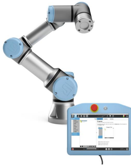
Fig 21. UR3e robotic arms with its teach pedant.
