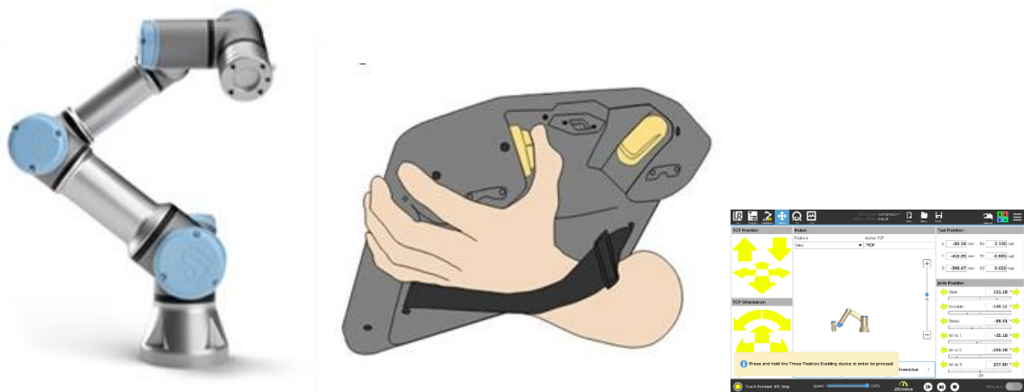
Figure 5.1 – UR3e collaborative robot and its Teach Pendant
