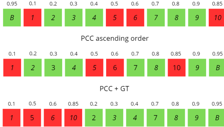
Figure 2.12. In this scheme the baseline heatmap is correctly classified, B has green colour. Above each heatmap there a hypothetic PCC value. Because the original image is correctly classified the PCC values are sorted in ascending order. Then all the heatmaps that are classified as GT are putted as last in the averaging order list.
