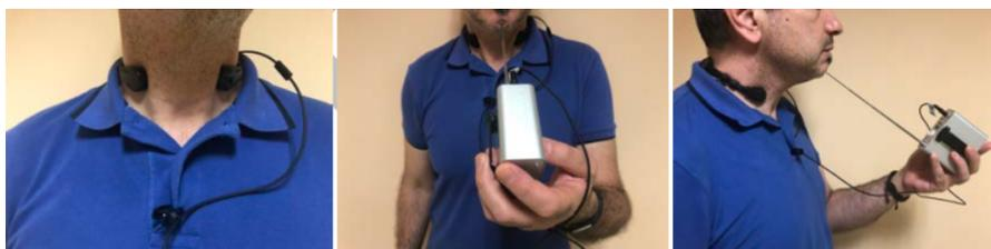
**Figure 2.4:** Correct positioning of the vocal Holter.[13]
