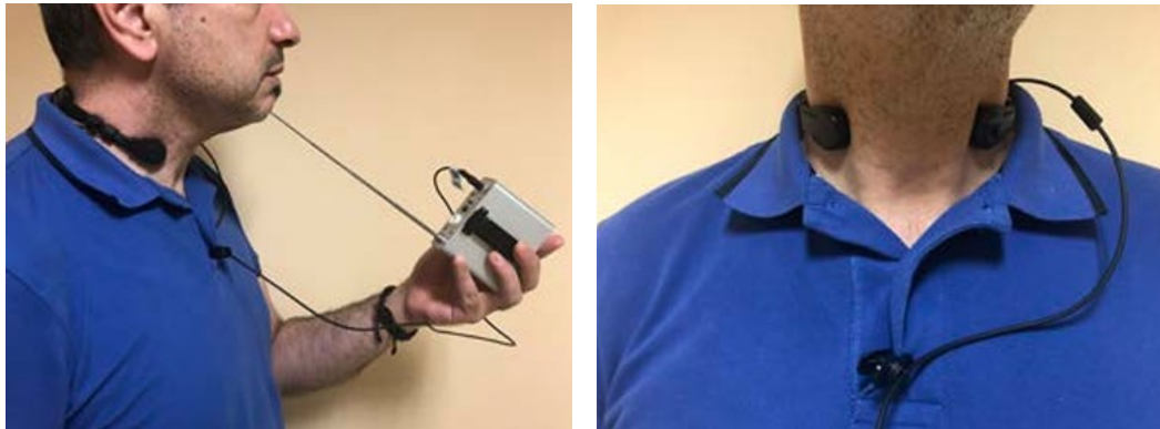
(a) Use of the telescoping antenna during the calibration of the contact microphone (b) Correct positioning of collar of contact microphone around the patient's neck
