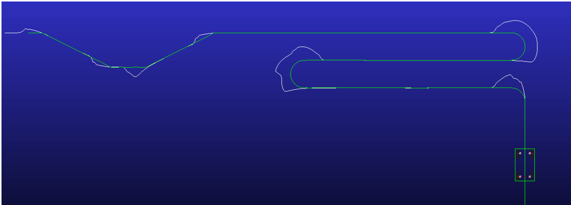
Figure 4.14: Trace of rear axle - Slip steering
