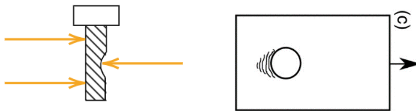
Figure 23 - Bearing Failure of Fastener and Plate
