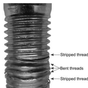
Figure 16 - Thread Failure during Tightening
