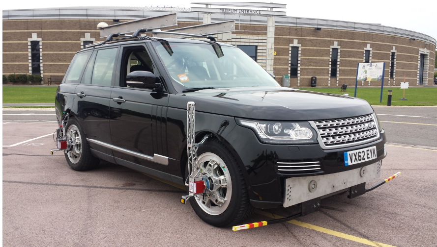
Figure 3.2: Wheel force transducer ( https://tyrecaenotebook.wordpress.com )
