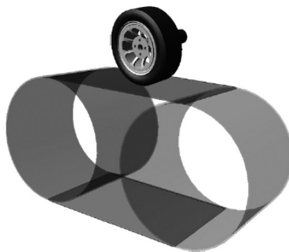
Figure 3.1: Belt tyre testing machine (Performance Vehicle Dynamics, 2018)
