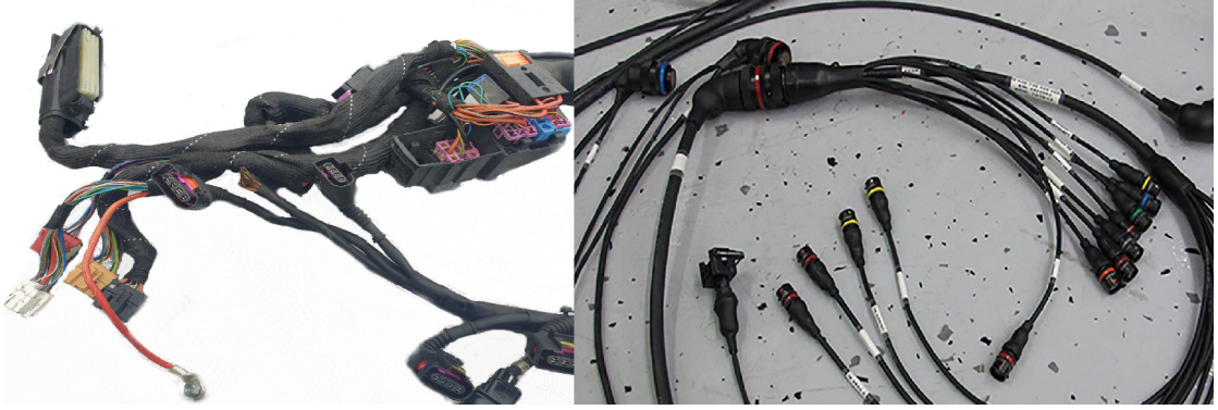
Figure 2.9: Commercial vs Motorsport Harness
