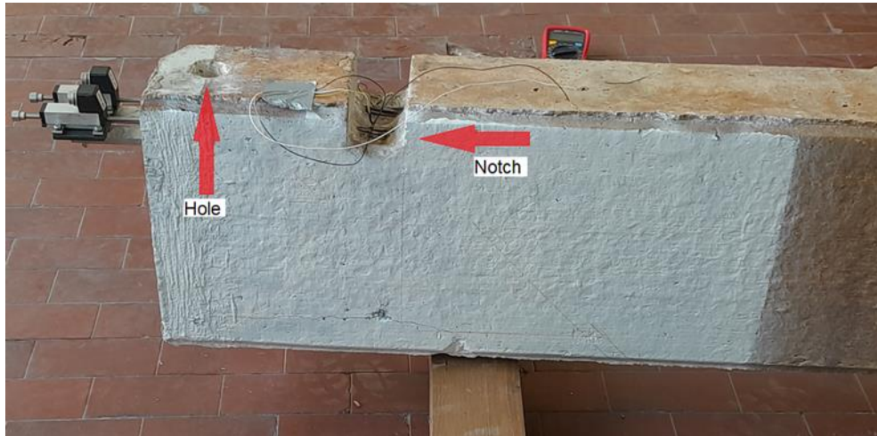
Figure 4-8 _ Notch at the bottom of beam _ Hole created to apply load
