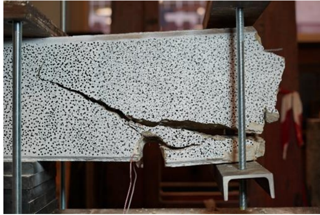
Figure 4-25 _ (a) Test 1, (b) Test 2, (c) Test 3 _ specimens after failure
