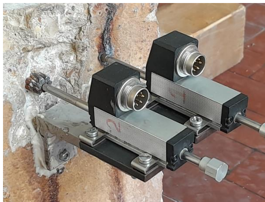
Figure 4-11 _ Gauges to record the relative slip of strand at the end of beam
