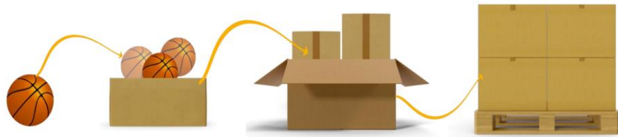
Figure 2.1.1: A four-layer packaging structure for warehousing applications
