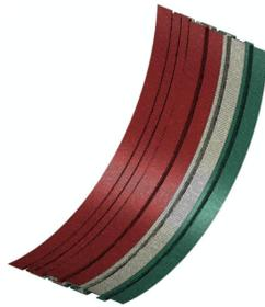
Figure 2.2.4: **Simplified FE-model of a flexible hose**[22].
