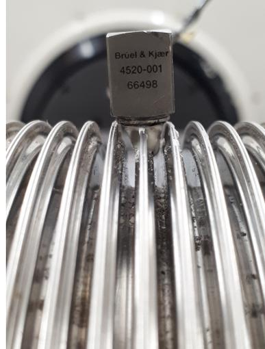
(b) Close-up at accelerometer attached directly to one convolution.
