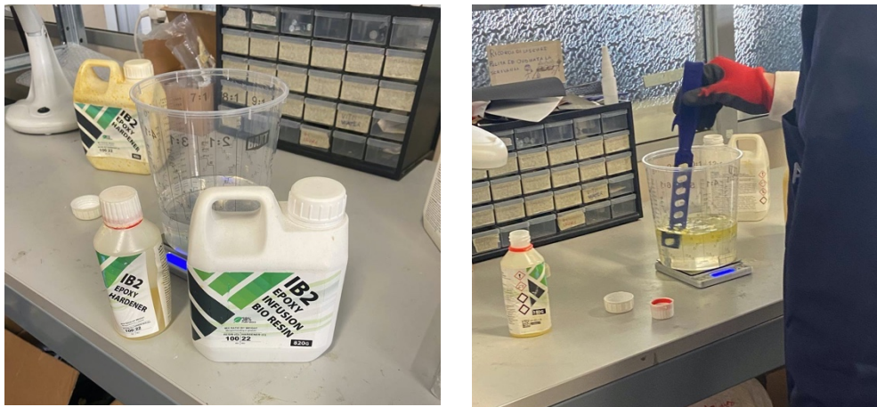
Figure 26: Mixing the resin with the hardener
