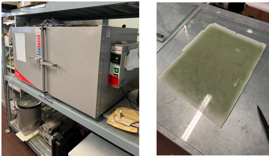
Figure 27: Curing oven (left) and final result of the lamination (right)
