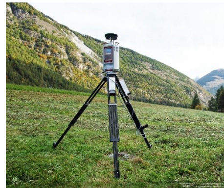
Figure 97 : TLS from https://geosurveyengineering.co.ke/terrestrial-laser-scanning/
