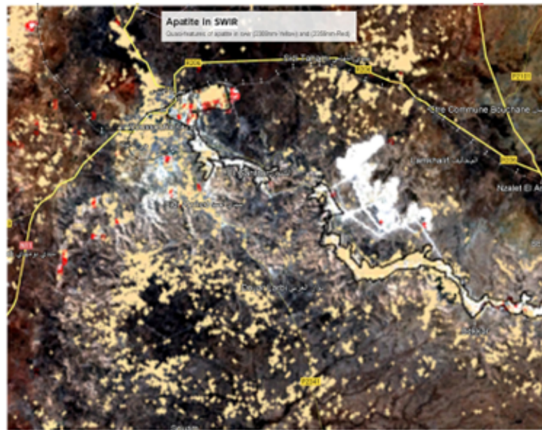
Mapping of Apatite in SWIR using EMIT sensor
