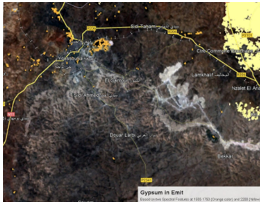
Mapping of Gypsum in SWIR using EMIT sensor
