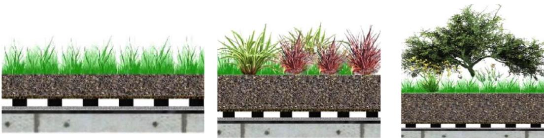
Figure 2. Classification of green roofs: extensive, semi-intensive and intensive (Besir & Cuce, 2018)
