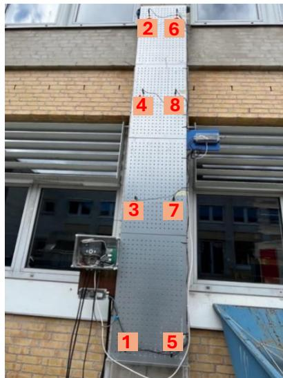
*Figure 7. Photo representing the system: the gutter, the 8-moisture sensor numerated and on the left the screen connected to the flow meter.*
