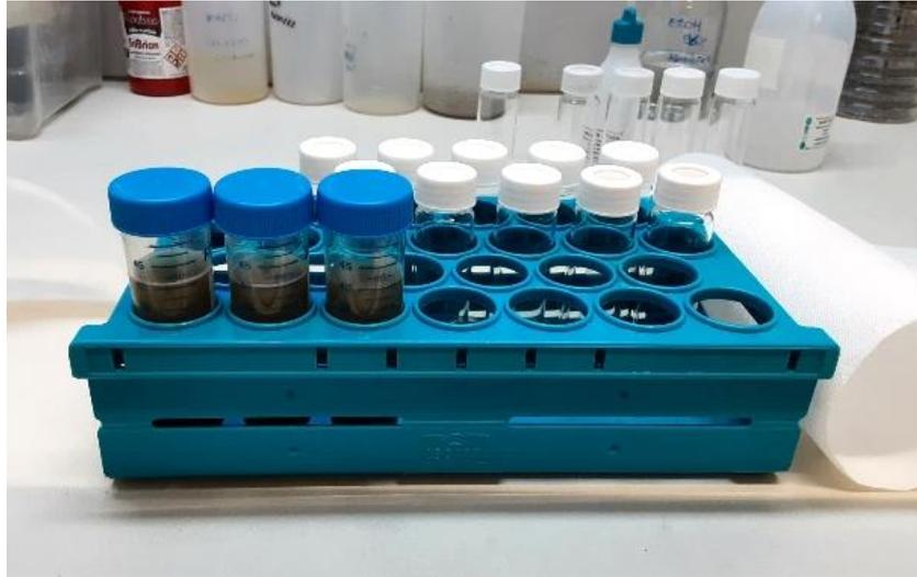
Figure 7. Falcon tubes and vials used for the characterization of the digestate
