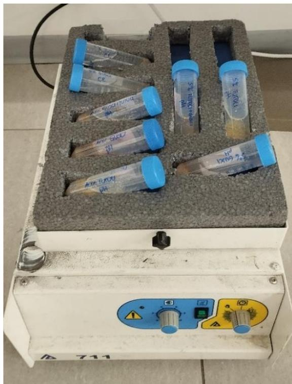
*Figure 10. Mixing of samples in Falcon tubes for 1 hour*
