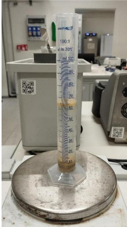
Figure 11. Graduated cylinder used for measuring bulk density
