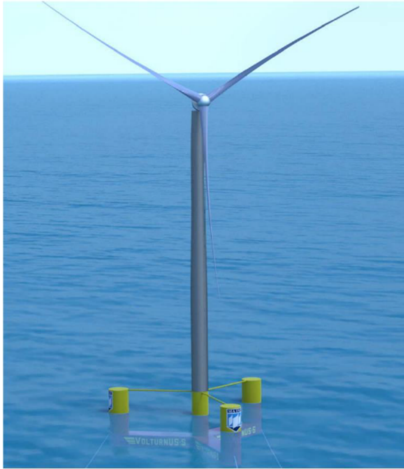
Figure 3.1: IEA-15-240 RWT and VoltornUS-S reference platform [4].
