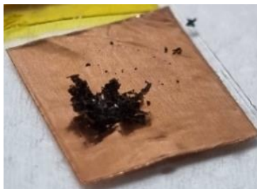
Figure 4.20: Sample reduced into powder placed on a copper substrate to minimize background signal and thermal energy accumulation. A cleaned spatula was used to reduce each sample into powder.
