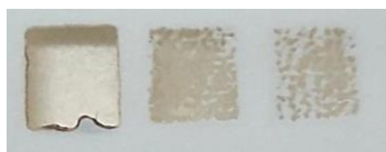
Figure 4.15: Untreated cellulose acetate membranes exposed to laser irradiation at different lasing powers. It is possible to notice how the obtained material is characterized by holes and, at excessive power (on the left), by brownish edges due to the ablation and combustion of the material.
