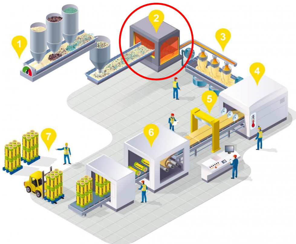
Fig.1 : Representation of the glass wool production process at Isover
