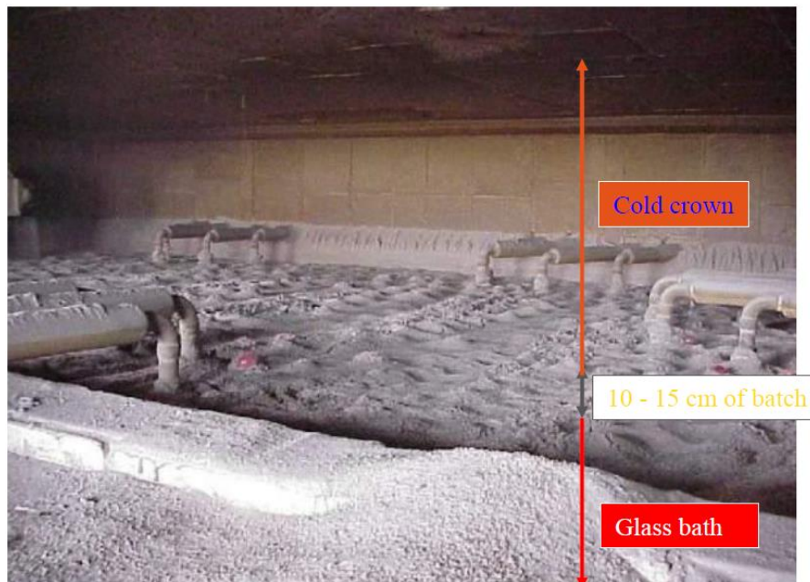
Fig.2 : Crown of an electrical furnace with top-electrodes [3]
