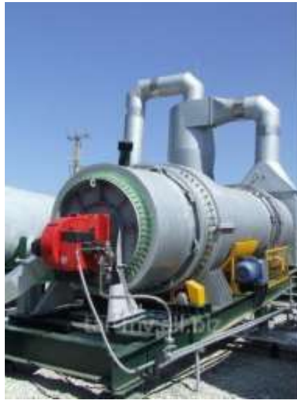
Figure No. 31: View of Thermal Desorption Plant (TDP)
