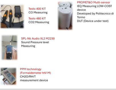
Reference Devices and DUT
