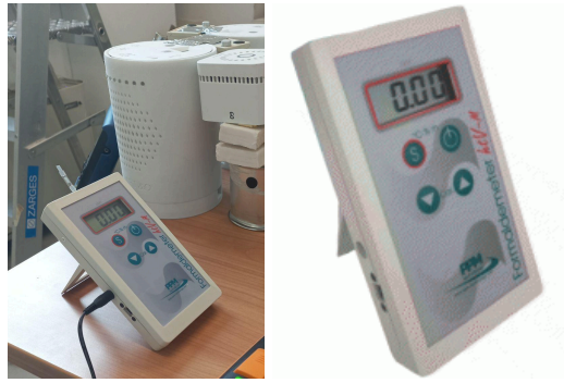
Fig. 13. The Formaldehyde measuring in the living lab (Second photo obtained from https://www.techrentals.com.my/PPM-HTV-M-Formaldehyde-Meter )
