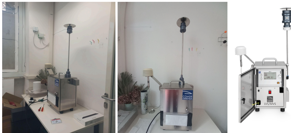
Fig. 12. The Particulate matter measuring in the living lab (Third photo obtained from https://www.j-aguirre-sl.com/en/product/particulate-matter-collection/ )
