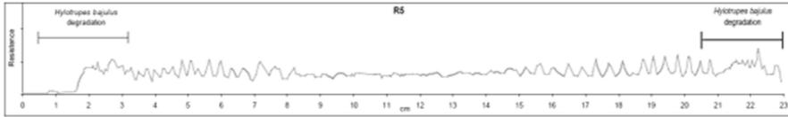
**Fig. 94/** example for Profile of the Resistograph® measurement in a degraded wooden piece. Source: Patricia C. et al., alNEGI, Faculty of Engineering, University of Porto, Rua Dr. Roberto Frias, 4200-465 Porto, Portugal. "Non-Destructive Structural Wood Diagnosis of a Medieval Building"
