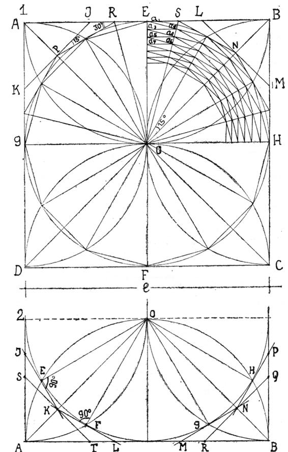
Fig. 30/ Longinoz Sumbadze, Construction of dodecagonal Gvirgvini on a square base, "The Architecture of the Georgian Folk Dwelling Darbazi", 1984
