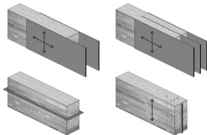
**Fig. 103/** Schematic example of FRP reinforcement using polymer rods and plates.
