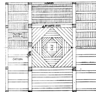
"The number of corbelling layers in both types varies according to region but is usually 5, 7, 9 or 10. The construction of the original form of the tüteklikli roof does not make use of nails." (Erarslan 2021, 8)
