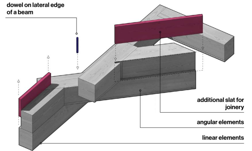
**Fig. 109/** Case study N4. Primary hall of Melikidze dwelling. Details of wooden frame in relation with masonry walls
