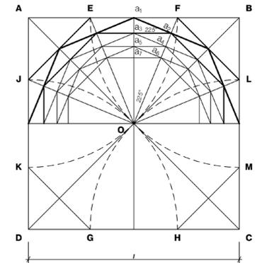
**Fig. 29/** Construction of octangular *Gvirgvini* with angular setting.
