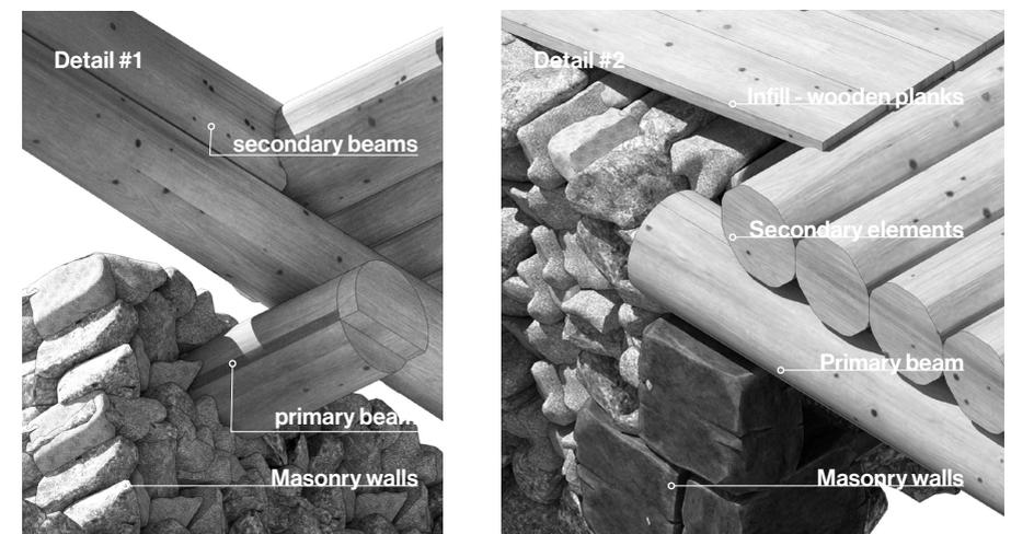
**Fig. 110/** Case study N4. Primary hall of Melikidze dwelling. Current state of the structure. Isometric scheme showing elements of primary Gvirgvini crown with typical decay and mechanical failure
