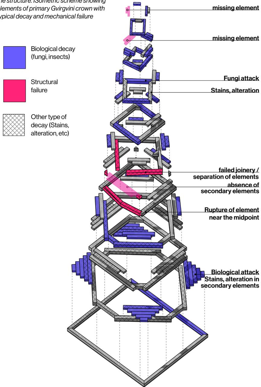
**Fig. 111/** Case study N4. Primary hall of Melikidze dwelling. Design state of the structure. Isometric scheme showing a proposal for substituted and restored elements of primary Gvirgvini crown
