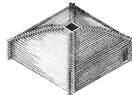
Fig. 5/ Reconstruction-of-Colchian-hut-according-to-Vitruvius-by-G.-Kipiani.jpg
