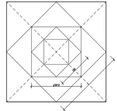
Fig. 27/ Quadrangular *Gvirgvini* of angular setting. Calculation of basic parameters
