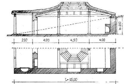
Fig. 11/ Longinoz Sumbadze, Darbazi with four-slated roof. Maximum slope of the terrain, "The Architecture of the Georgian Folk Dwelling Darbazi", 1984.
