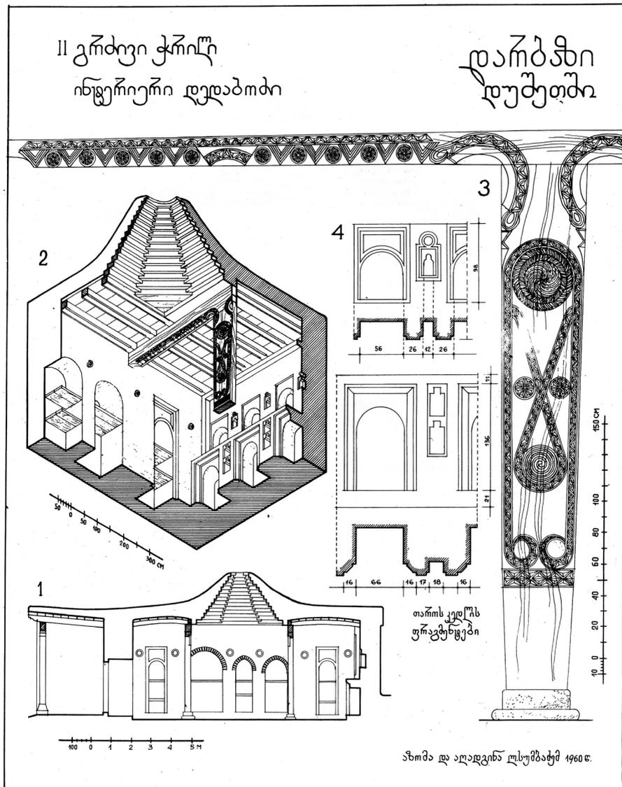
**Fig. 9/** Longinoz Sumbadze, Darbazi according to the measurements and reconstruction by L. Sumbadze, longitudinal section (1), interior (2), Deda-bodzi with the Tavkhe beam (3), fragments of the niches (4), "The Architecture of the Georgian Folk Dwelling Darbazi", 1984.
