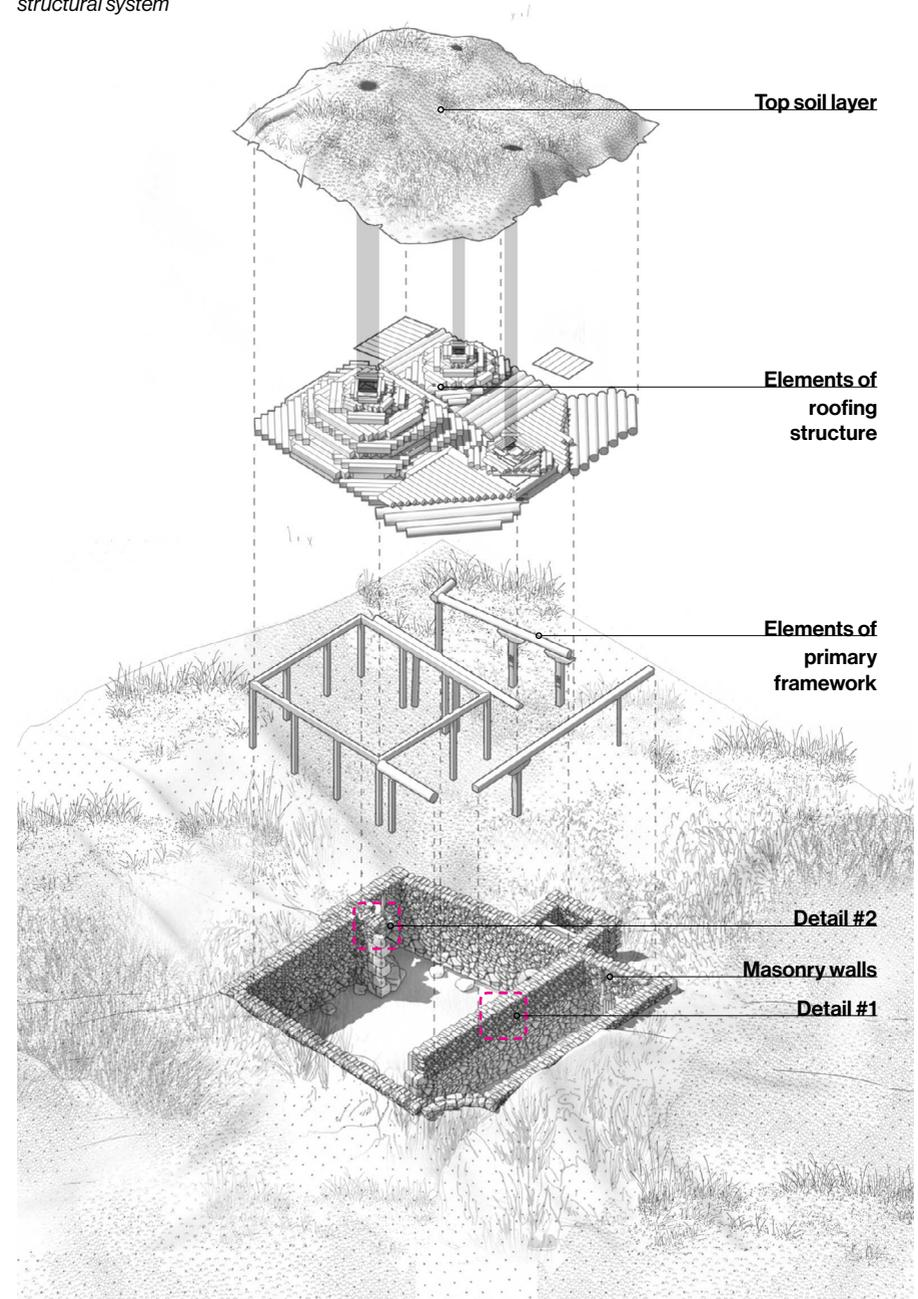
**Fig. 107/** Case study N4. Primary hall of Melikidze dwelling. Construction detail of Gvirgvini crown, showing the main components
