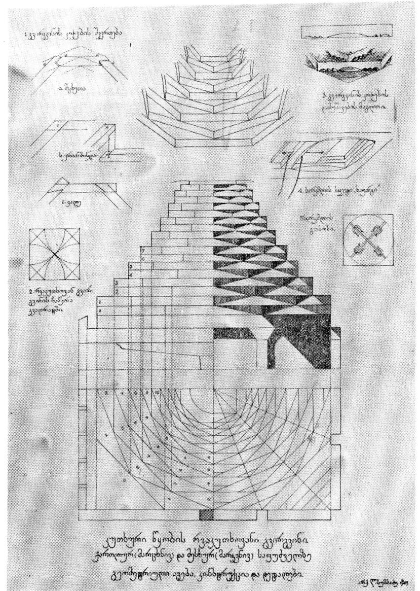
**Fig. 21/** Longinoz Sumbadze, Octangular Gvirgvi of angular setting. Geometric structure, construction and details based on Kartlian (left) and Meskian (right) methods, "The Architecture of the Georgian Folk Dwelling Darbazi", 1984
