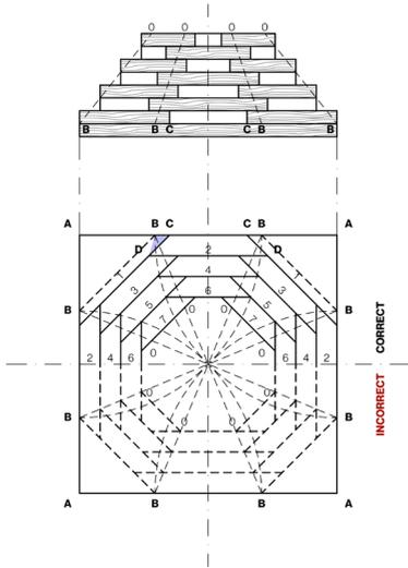
“Field observations convinced us that the edges of *Gvirgvini* appear correct when the imaginary borderlines of BO, connecting the polyhedron B corners with the center of *Gvirgvini*, pass through the intersection midpoints of DC lateral beam edges” (Sumbadze [1984], [59], translated by Gvantsa Tskipurishvili)
