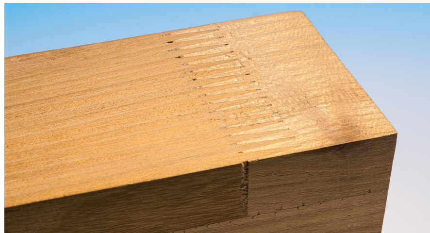
Fig 51 – Robinia wood as highly resistant glued laminated timber. Source – Fraunhofer Institute for Wood Research, Wilhelm-Klauditz-Institut WKI, 2022. https://www.wki.fraunhofer.de/en/research-projects/2022/ROB-INIA_glued-laminated-timber-made-from-robinia.html
