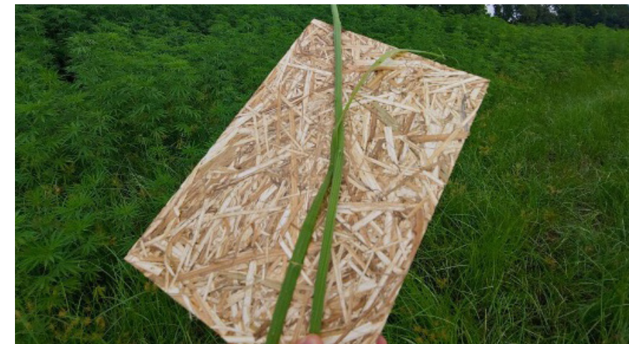
Fig 62 – OSB board made with 94 – 97% hemp fibres and 3 – 6% formaldehyde-free Resin. Source – Plantd Materials. https://www.plantdmaterials.com/product
