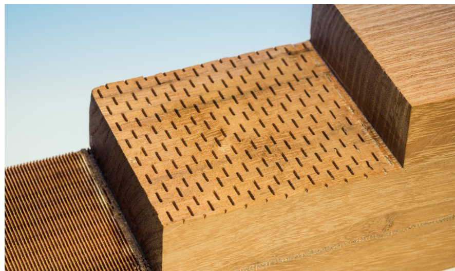
Fig 52 – Surface structuring by means of lasers improves the bonding of the boards. Source – Fraunhofer Institute for Wood Research, Wilhelm-Klauditz-Institut WKI, 2022. https://www.wki.fraunhofer.de/en/research-projects/2022/ROB-INIA_glued-laminated-timber-made-from-robinia.html
