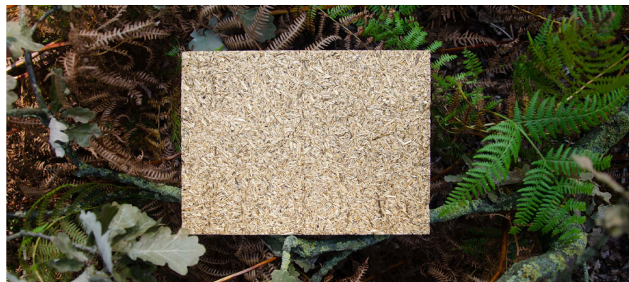
Fig 79 – Compost board panels made from agricultural residual fibres. Source – COMPOST BOARD, Rikaalsmeer. https://www.compostboard.bio/services/
