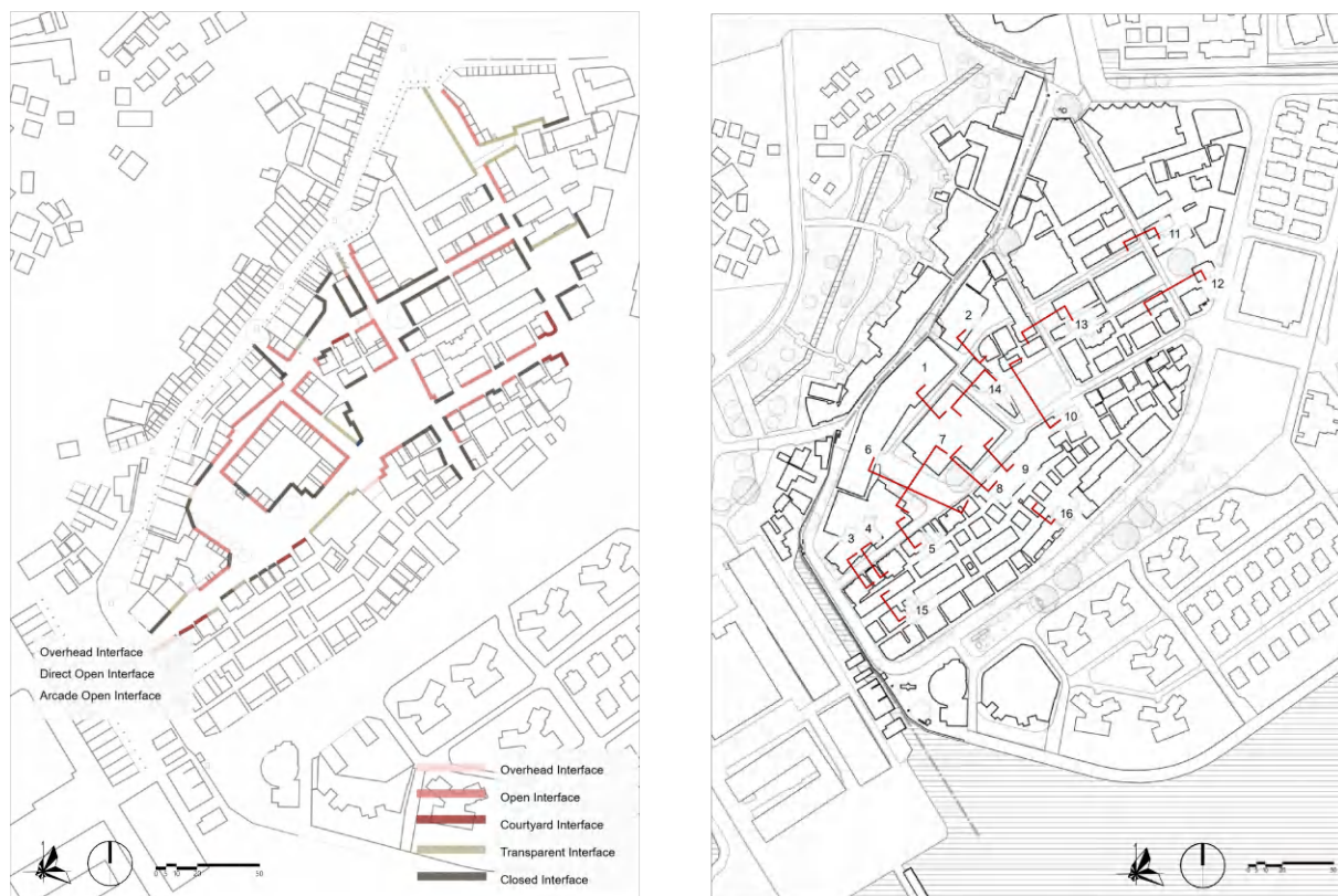
Figure 3-11 Types and Distribution of Living Street Interface Spaces (Source: Drawn by the Author)
