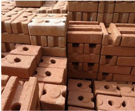
Figure 4.54 Compressed Earth Blocks-
