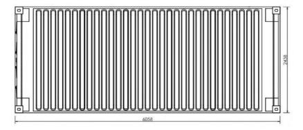
Figure 135: 20ft Shipping container - roof plan
