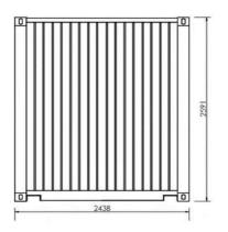
Figure 136: 20ft Shipping container - front elevation
