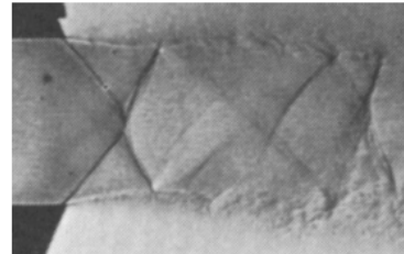
Figure 2.7: Shocks Interaction of Opposite Family - Overexpanded Nozzle
