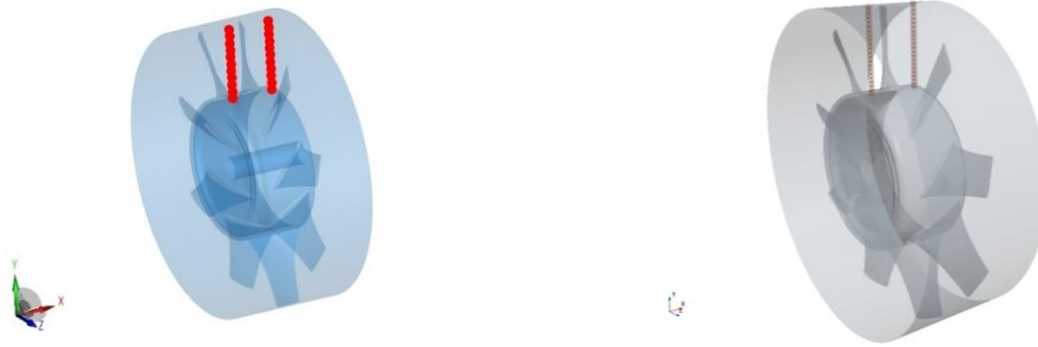
Figure 5.20: Line probes position for estimation of Axial velocity along the blade radius (FIRE M left, Star-ccm+ right)
