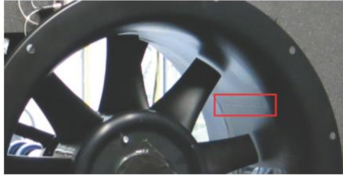
Figure 4.3: Wall pressure transducers
