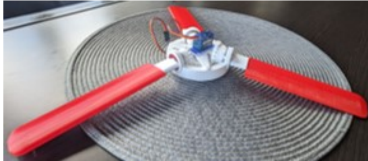
Figure 1.7: Proposed design of a controllable pitch Smart Boomerang
