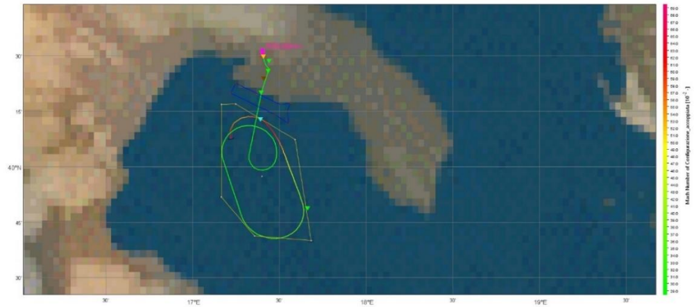
Figure 4.26: ASTOS output for the trajectory related to the descent and landing phases of WhiteKnightTwo depicted on the 2D map for the mission scenario with the release phase directed towards Taranto
